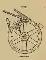
lower part of the thread-layer stop H at each side of the machine; when the coverer slides are in position to be shogged, the pin B abuts against their side and pushes them along the slide-bar
